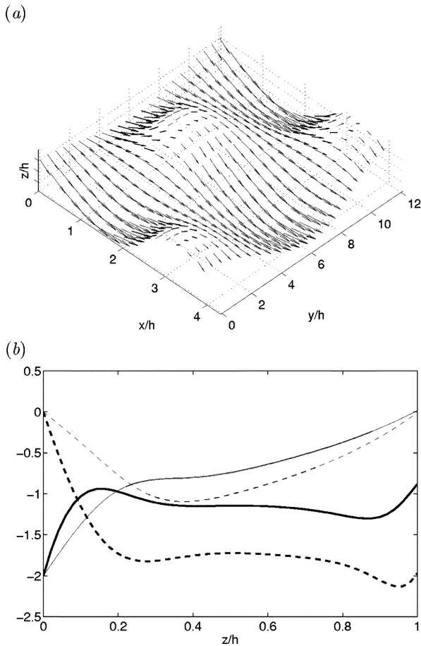
FIG. 4. (a) Film surface and surface velocity field for flow down a three-dimensional corrugated wall. (b) Profiles of functions  $f'(\tilde{z})$  (thick lines) and  $r(\tilde{z})$  (thin lines). The imaginary parts are shown as dashed lines.
