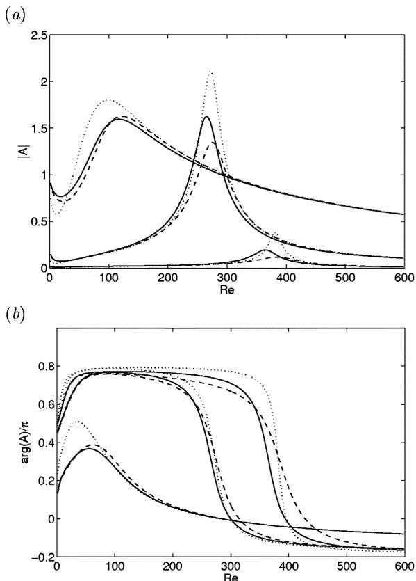
FIG. 2. (a) Surface amplitude and (b) phase shift of a water film down a two-dimensional corrugated wall for  $l=0.001$  m (right),  $0.002$  (middle),  $0.005$  (left), and  $Ma=0$  (dotted lines),  $0.1$  (dashed lines),  $1$  (solid lines).
