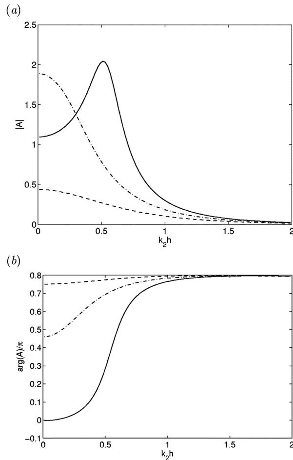
FIG. 3. (a) Surface amplitude and (b) phase shift of film flow down a three-dimensional wavy wall for  $\text{Re}=225$  (dashed lines),  $270$  (dashed-dotted lines), and  $300$  (solid lines).
