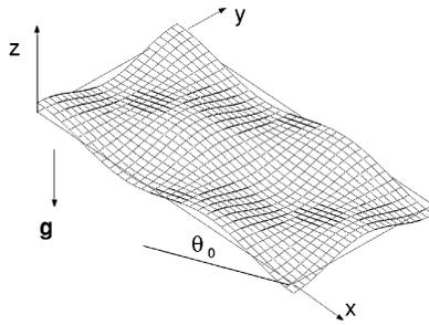
FIG. 1. Schematic illustration of film flow down an inclined wall with three-dimensional periodic corrugations.
