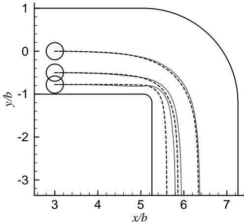
Figure 3: The effect of the initial position,  $h_1/b$ , on the particle trajectory for  $a/b = 0.2$  and  $E_0^* = 5$ . Dashed lines represent results found using the BEM, and the solid lines represent the prediction by the PDM.
