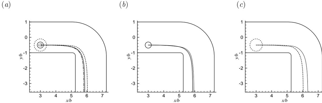
Figure 4: The effect of the particle size,  $a/b$ , on the particle trajectory for the case of  $h_1/b = 0.5$  and  $E_0^* = 5$ . Dash-dotted, solid (thick), and dashed lines represent  $a/b = 0.1, 0.2$ , and  $0.4$  respectively in (a). In (b-c) the thin-solid line represents the estimate from the PDM.
