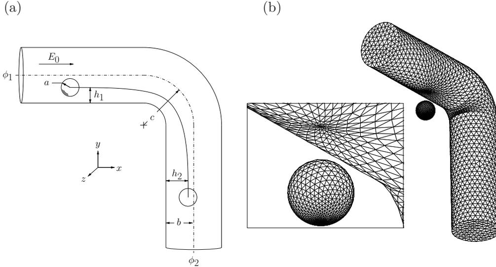
Figure 1: (a) Schematic of a non-conducting particle moving through a cylindrical pore. (b) The adaptive mesh (note that the particle is translated outside for better visualization).
