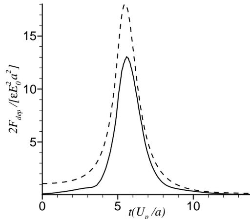
Figure 5: The normalized DEP force as the particle moves along the trajectory shown in Figure 4(c) from the BEM simulation (dashed line) and the point-dipole estimate (solid line).
