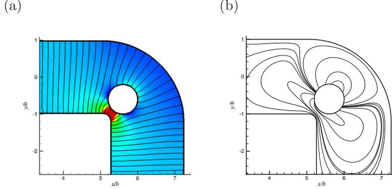
Figure 2: (a) Equipotential contours plotted over the electric field strength and (b) flow streamlines around a particle ( $a/b = 0.4$  and  $\zeta_w = 0$ ) positioned close to the inner wall.
